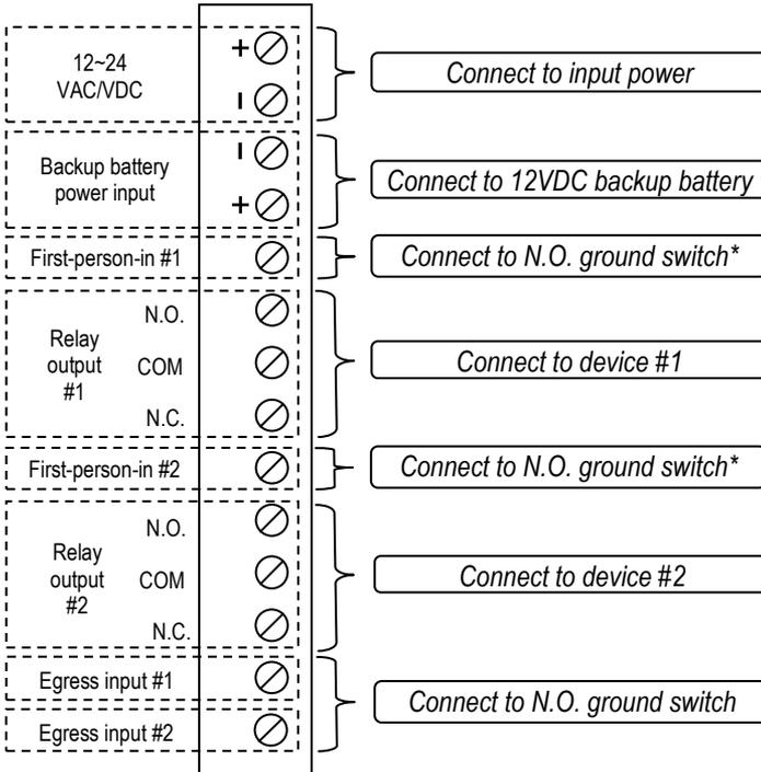
\* When the optional N.O. switch is activated, the first-person-in function suspends the operation of the SA-027HQ annual timer. If a relay is turned on before the first-person-in feature is activated, the relay will remain on until the first-person-in feature is deactivated. Once deactivated by turning the switch off, the timer will turn on the last programmed function prior to the first-person-in activation.
